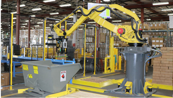
The parcel robotic sortation system uses a robot that operates inside a cell, along with a conveyor and autonomous mobile robots.
