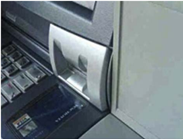
A fake reader has been placed on top of the machine's authentic slot.
