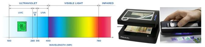
**Shortwave UV** light extends from 180 to 280 nm with a peak in energy at about 254 nm. For best results the shortwave UV source should be appropriately filtered (not unfiltered). Ultraviolet equipment that produces light in the shortwave region is typically used for toxicology, fluorochemistry, and germicidal applications.
